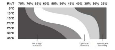
The diagram is based on the assumption that temperatures >=20 °C are for living quarters and temperatures <=20 °C are for basement quarters.
