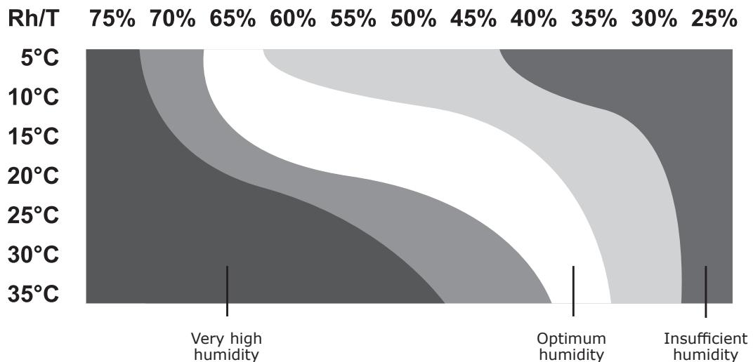
The diagram is based on the assumption that temperatures  $\geq 20^{\circ}\text{C}$  are for living quarters and temperatures  $\leq 20^{\circ}\text{C}$  are for basement quarters.
