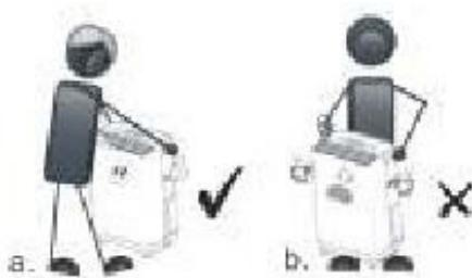
Place face to the front of the unit and lift it when move the machine.
