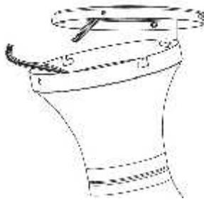
**2.** Lift the fan assembly and hand onto the hook on mounting bracket. This will permit you to make the electrical connections without having to hold the fan up as well.
